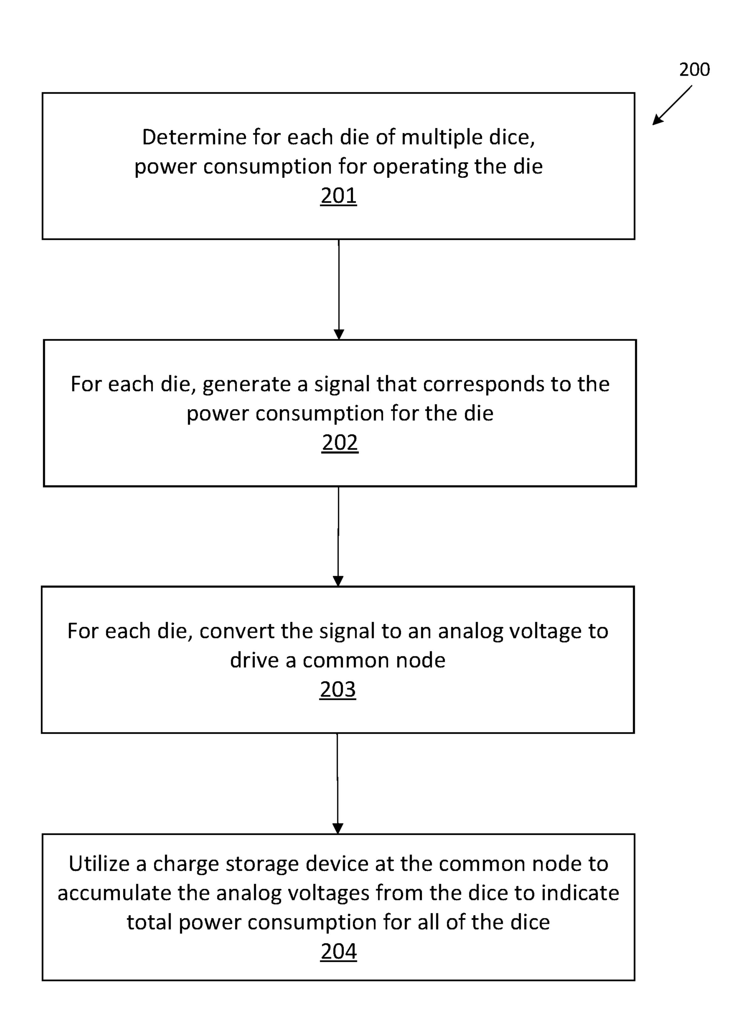
Monitor at a common node shared by multiple dice, accumulated voltage that indicates total power consumption for all of the dice, where each die generates a signal that corresponds to power consumption for the die, converts the signal to an analog voltage to drive the common node, and a charge storage device at the common node accumulates the analog voltages from the dice
