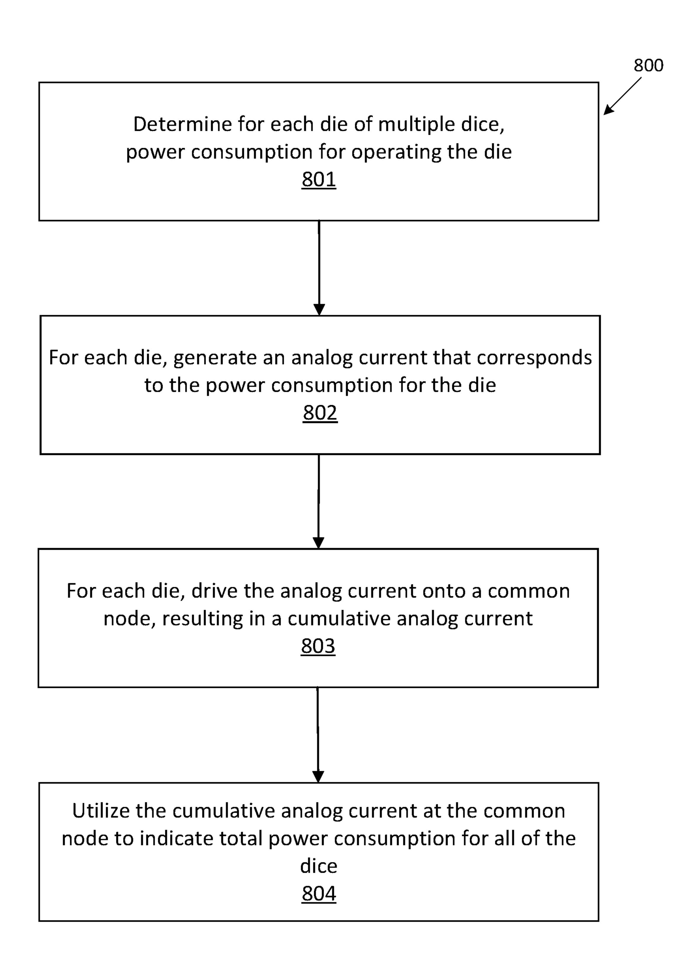
Monitor at a common node shared by multiple dice, a cumulative analog current, where each die generates an analog current that corresponds to power consumption for the die and drives the analog current onto the common node, and where the cumulative analog current at the common node indicates total power consumption for all of the dice
