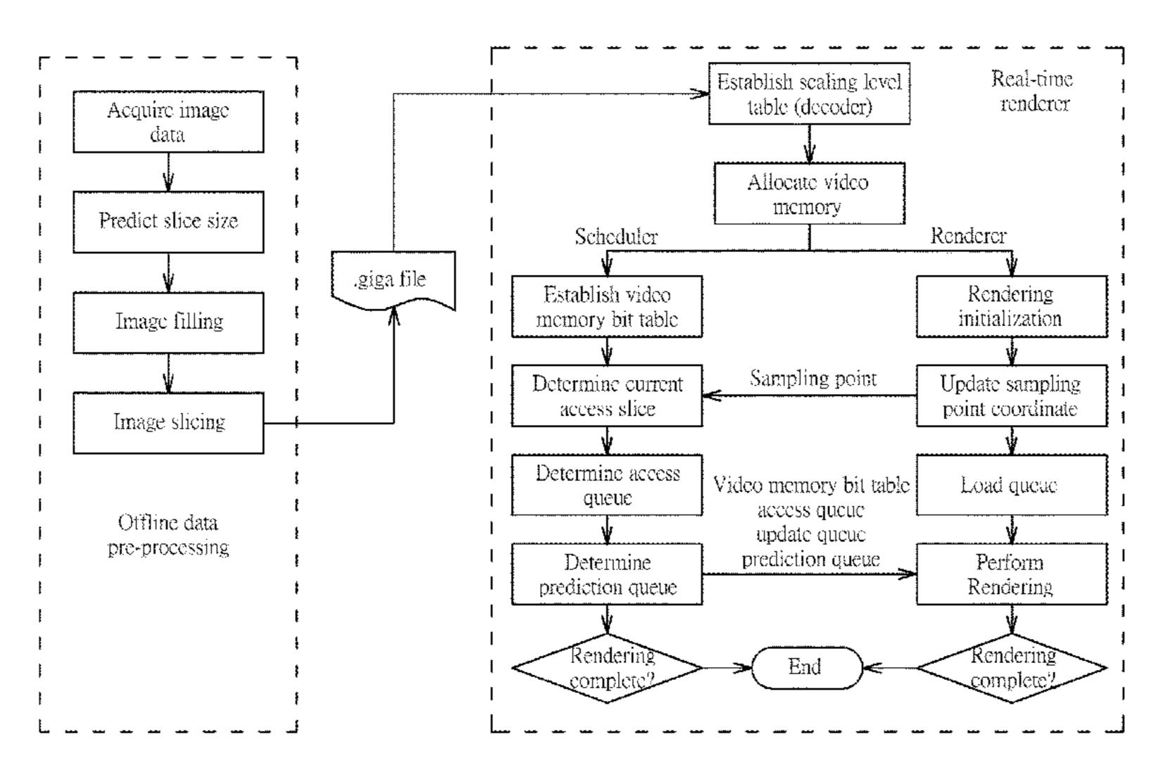
giga-pixel images. The present invention may render an image originally requiring a 40G or more video memory capacity on a common video card with a 1G-4G video memory capacity.
