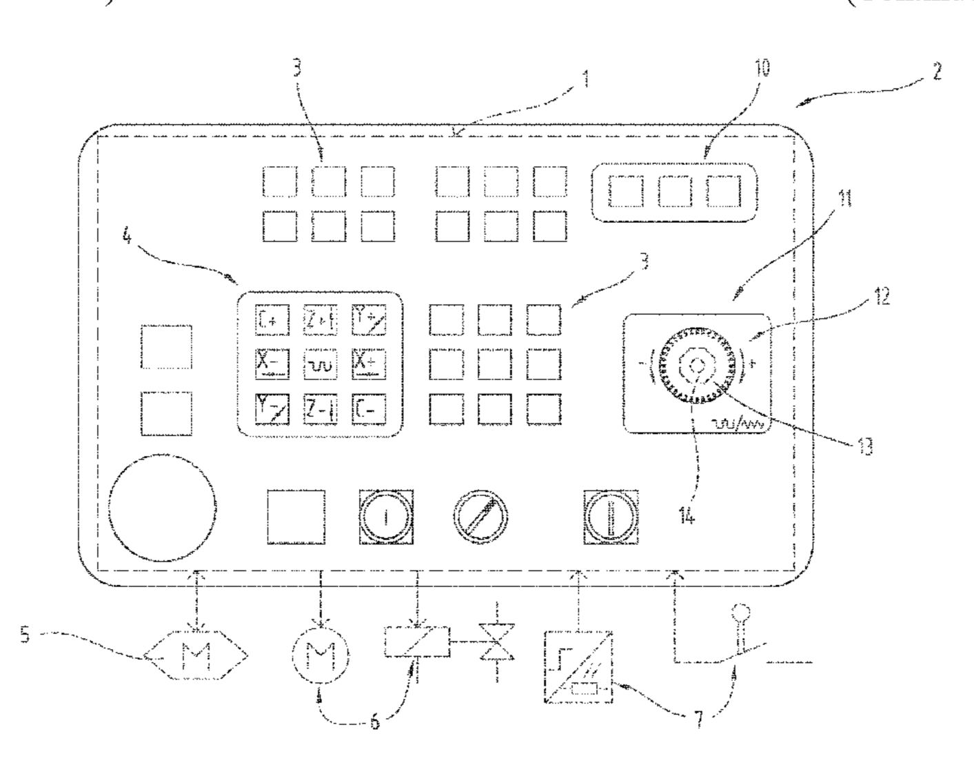
traverse rate during a rapid-traverse phase of the tool head. The multi-functionally designed operating element is designed as a rotary actuator operating element comprising a continuously rotatable actuating member.
