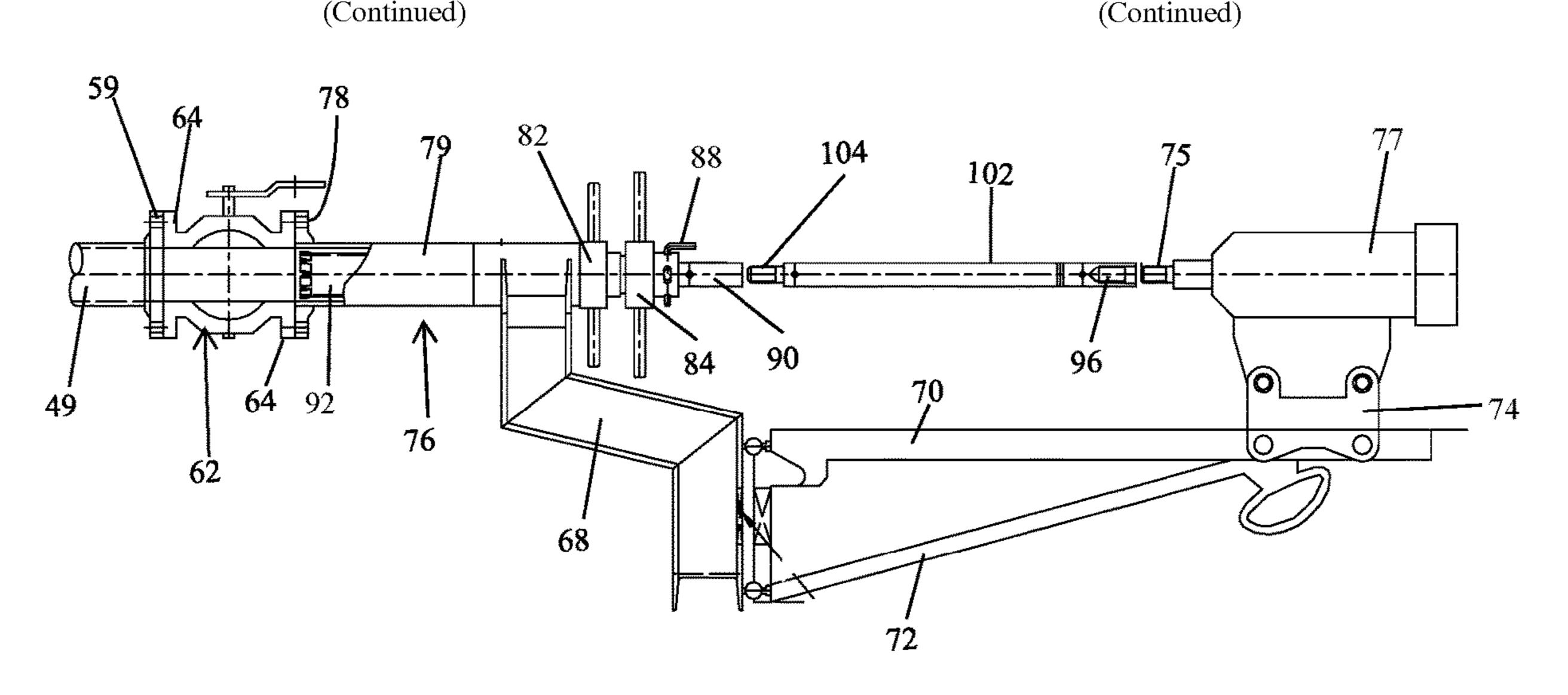
lance. The method further comprises (c) retracting the tool from the solids injection lance and the supply line section. Also disclosed is an apparatus for removing a blockage in a solids injection lance extending into a direct smelting vessel.
