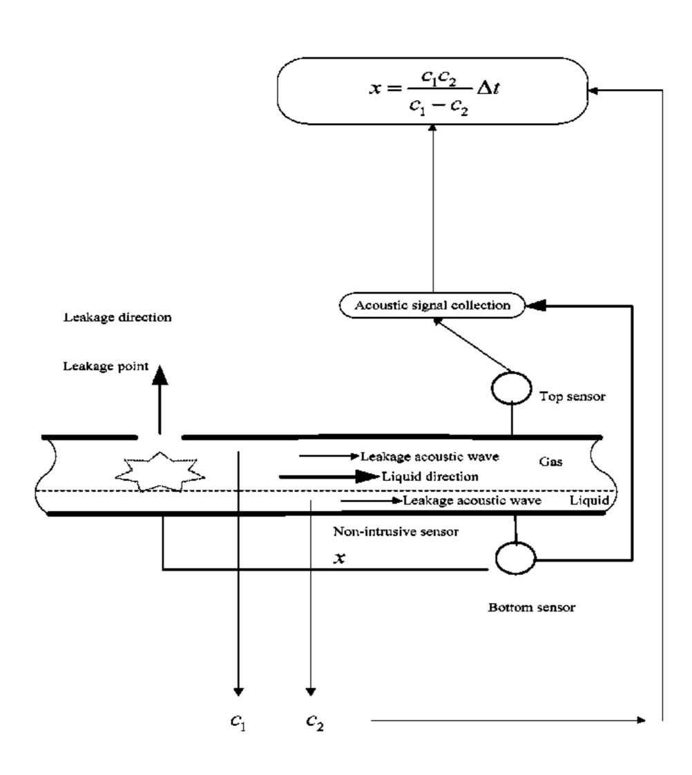
the acoustic velocity in a gas and the time difference into the single-point dual sensor-based leakage formula. The installation of sensors at two ends of a pipeline, avoids missing detection of leakage acoustic wave signals by a single sensor, reduces the number of installed sensors, and is low in cost, high in safety and strong in applicability to a gas-liquid stratified flow pipeline.
