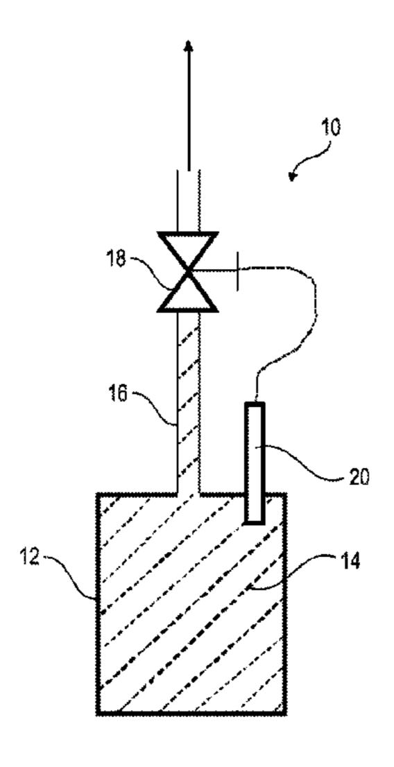
fuel under an upwardly limited pressure; opens the discharge line if the vaporous fuel has been detected and blocks the discharge line if no vaporous fuel has been detected; and discharges the vaporous fuel through the opened discharge line while retaining the liquid fuel.
