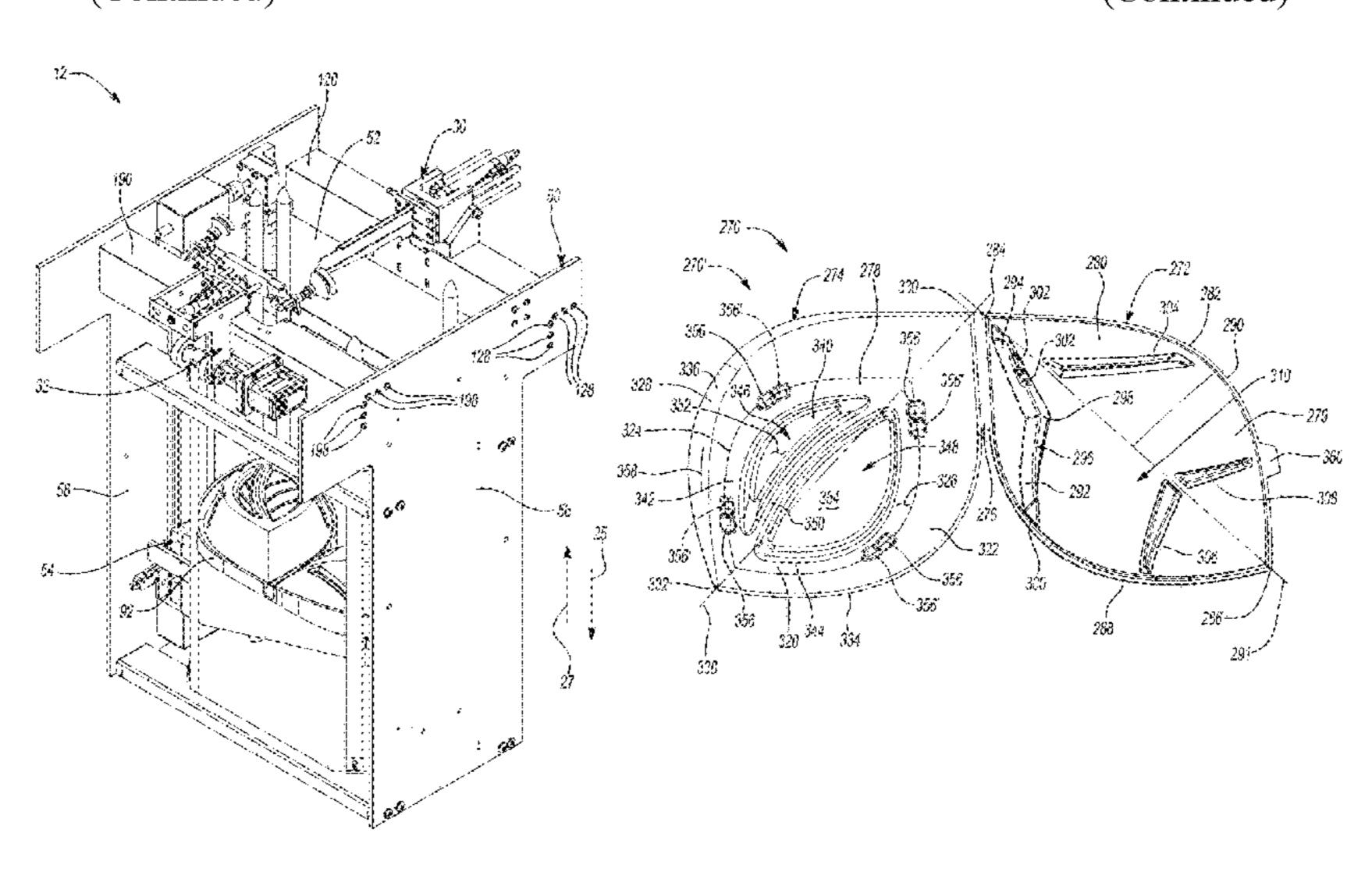
housing in a first direction and a second direction opposite the first direction. The transfer subassembly is coupled to the housing and disposed at least partially within the inner area. The transfer subassembly includes a vacuum suction cup. The vacuum suction cup is configured to operatively engage a first box of the plurality of boxes to remove the first box from the stack and pivot the first box about a rotational axis to a surface outside of the inner area.
