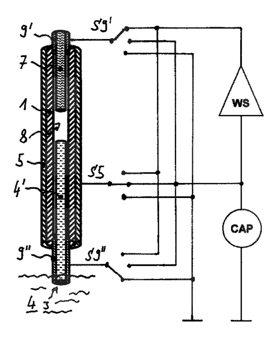
with the working fluid, the first electrical contact can be electrically connected to the measuring unit via a low-resistance converter circuit.
