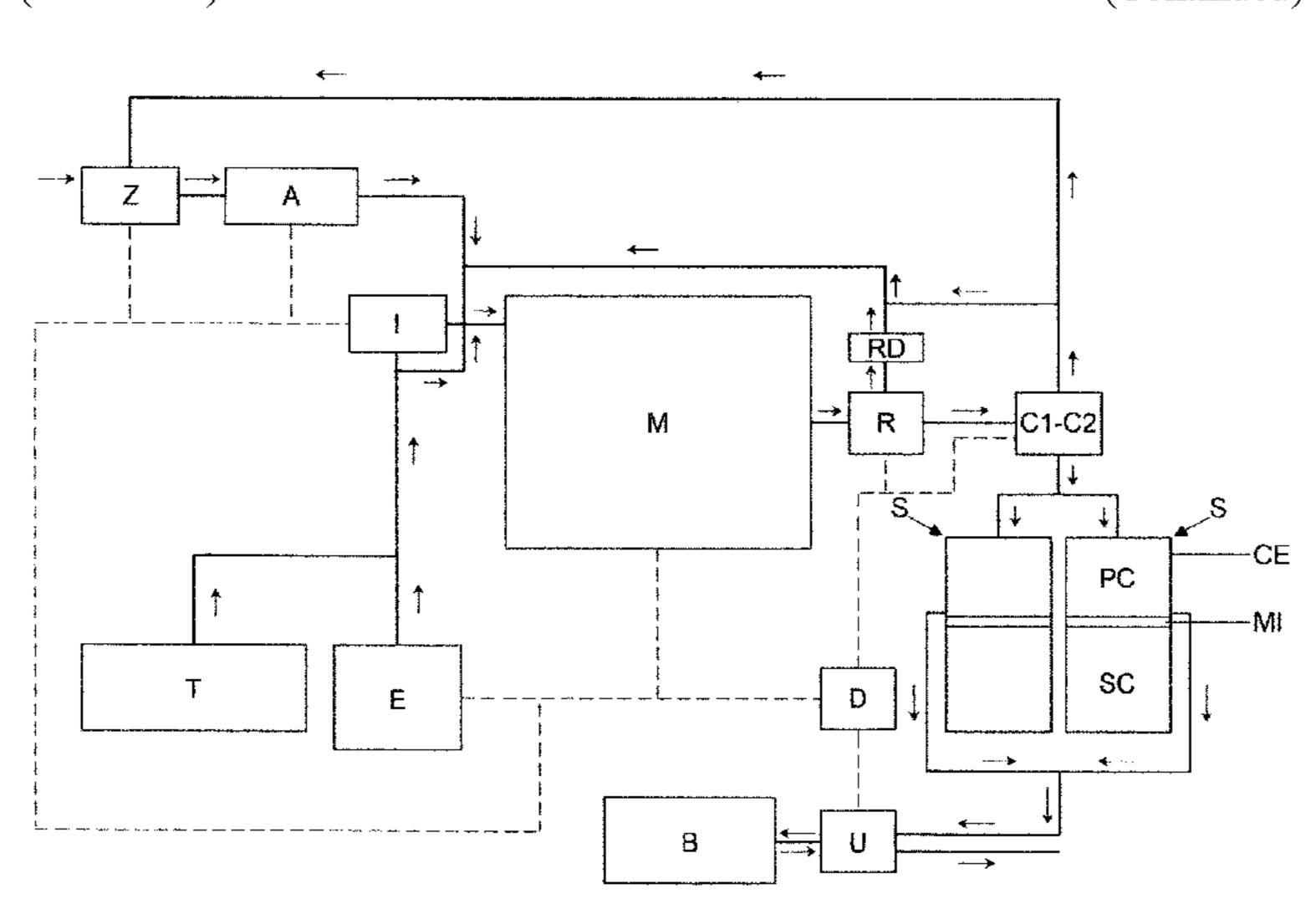
exhaust gases reintroduced into said combustion or reaction chambers of said endothermic engines M; —Means C1 and C2 for filtering the exhaust gases released from endothermic engines M, and supplied by means R; —Means S for confining the polluting substances obtained from the filtering of said exhaust gases released from said endothermic engines M, supplied by said means R.
