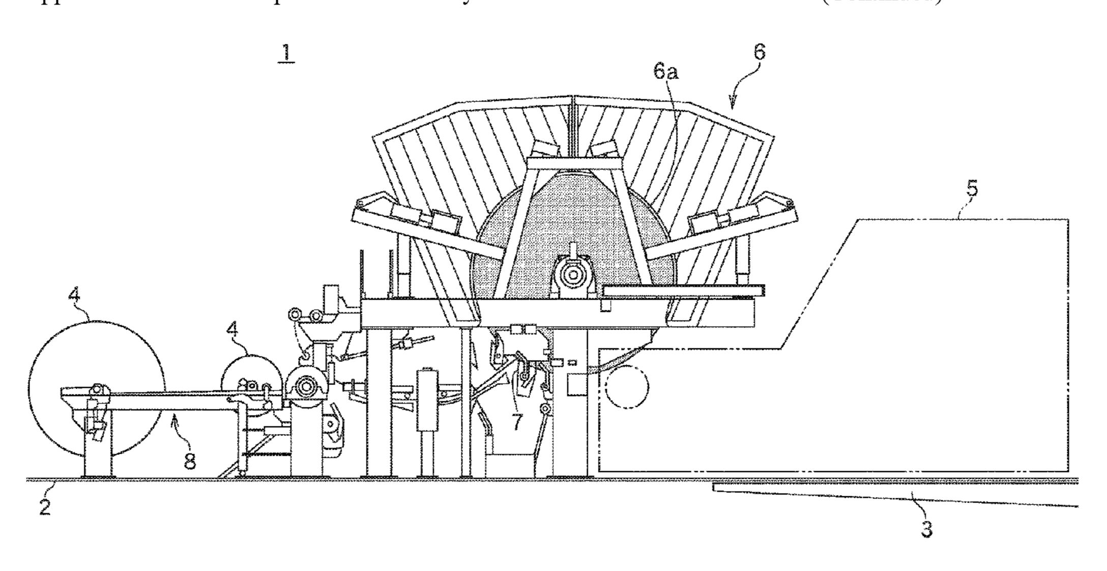
the first sheet-forming machine. The winder 8 winds up the dry paper material at a speed corresponding to the sheet-forming speed of the first sheet-forming machine or to the sheet-forming speed of the second sheet-forming machine to form the paper roll material.
