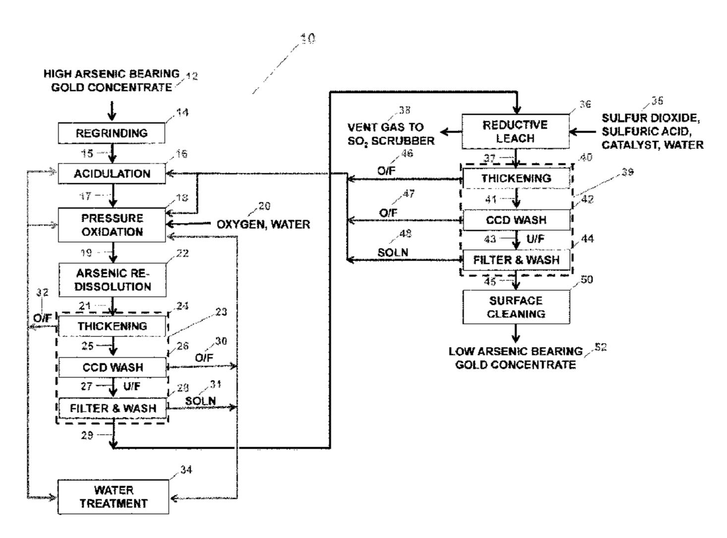
process may further comprise reacting the first washed slurry/solid with sulfur dioxide in a reductive leach step, and applying a second solid/liquid separation and wash step to form a second washed slurry/solid and second acid-containing solutions. The second washed slurry/solid may be a low arsenic-bearing gold concentrate.
