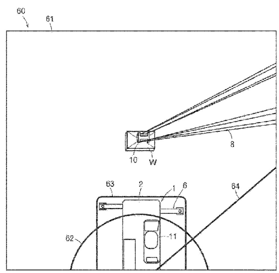
boundary which is a boundary between a range where the hook may move, and a range where the hook may not move, in a direction approaching the vehicle. The display device displays an image wherein images indicating the inner boundary are superimposed on the image photographed with the camera.
