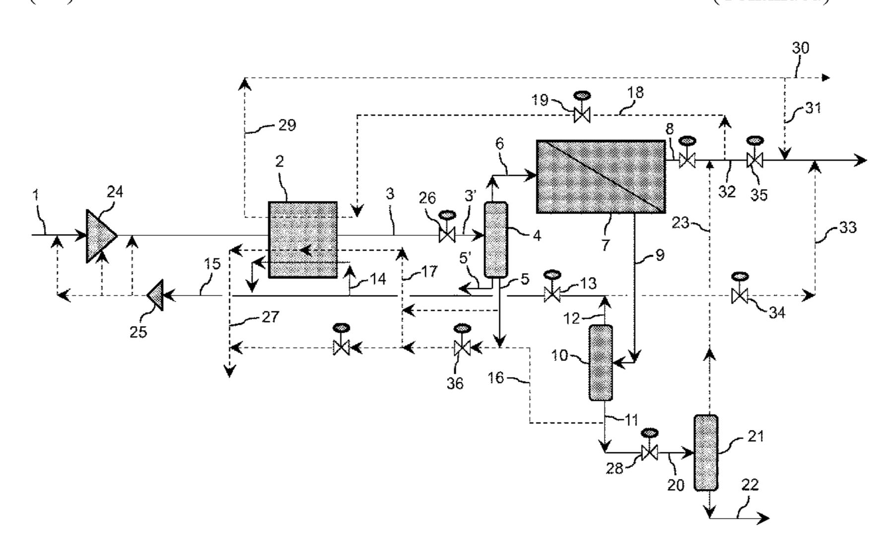
a second phase separator vessel to produce a liquid stream and a gas stream; step e): introducing at least one portion of the liquid stream resulting from step d) into a JT expansion means; step f): heating at least one portion of the expanded by introduction into the heat exchanger used in step a) counter-current to the feed stream.
