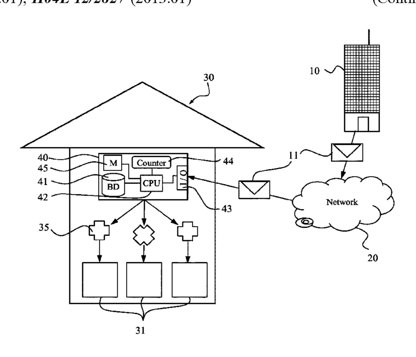
default power mode. If another authentic secured control message has been received, then returning to the step of initializing the counter.
