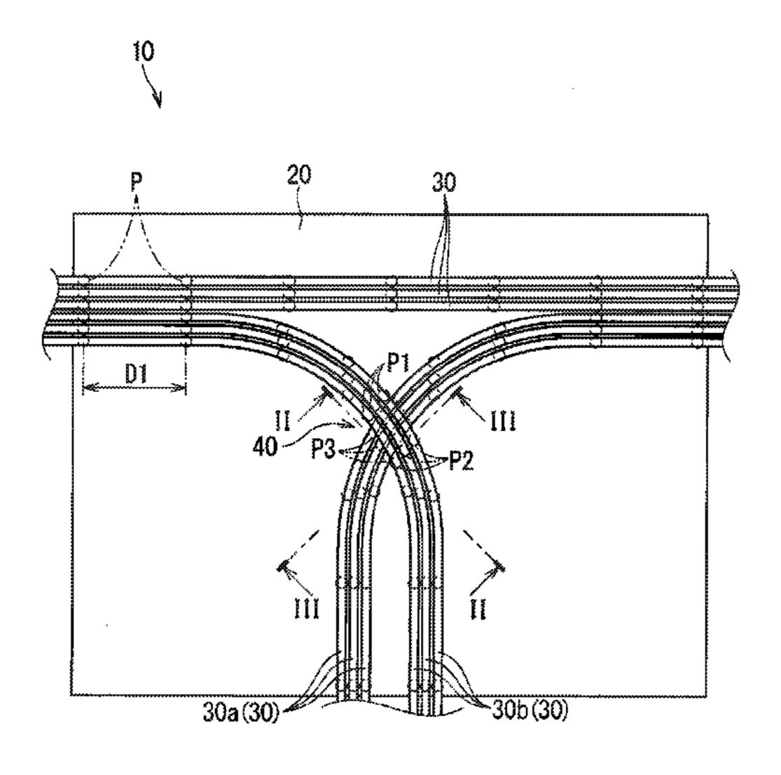
a thickness of at least one of the insulating covering of the lower wiring part and the sheet material in the position is reduced.
