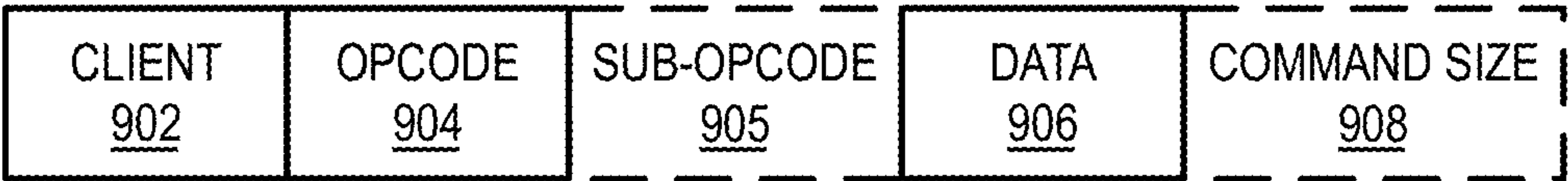
FIG. 9A GRAPHICS PROCESSOR COMMAND FORMAT 900
