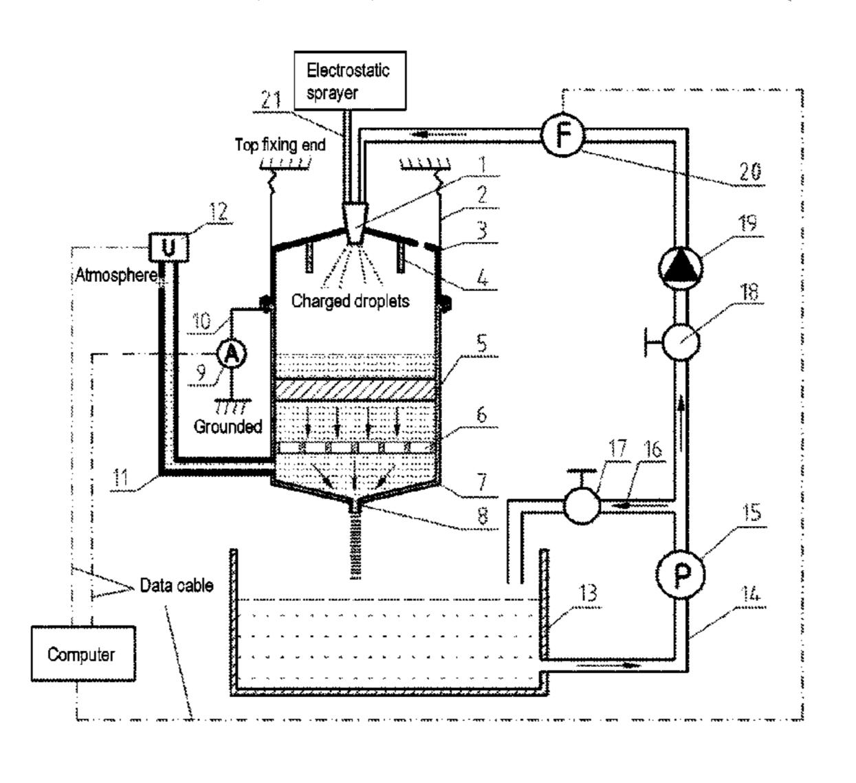
storage tank to the electrostatic atomization nozzle. Measurement data of the ammeter is acquired and processed by a computer in real time.
