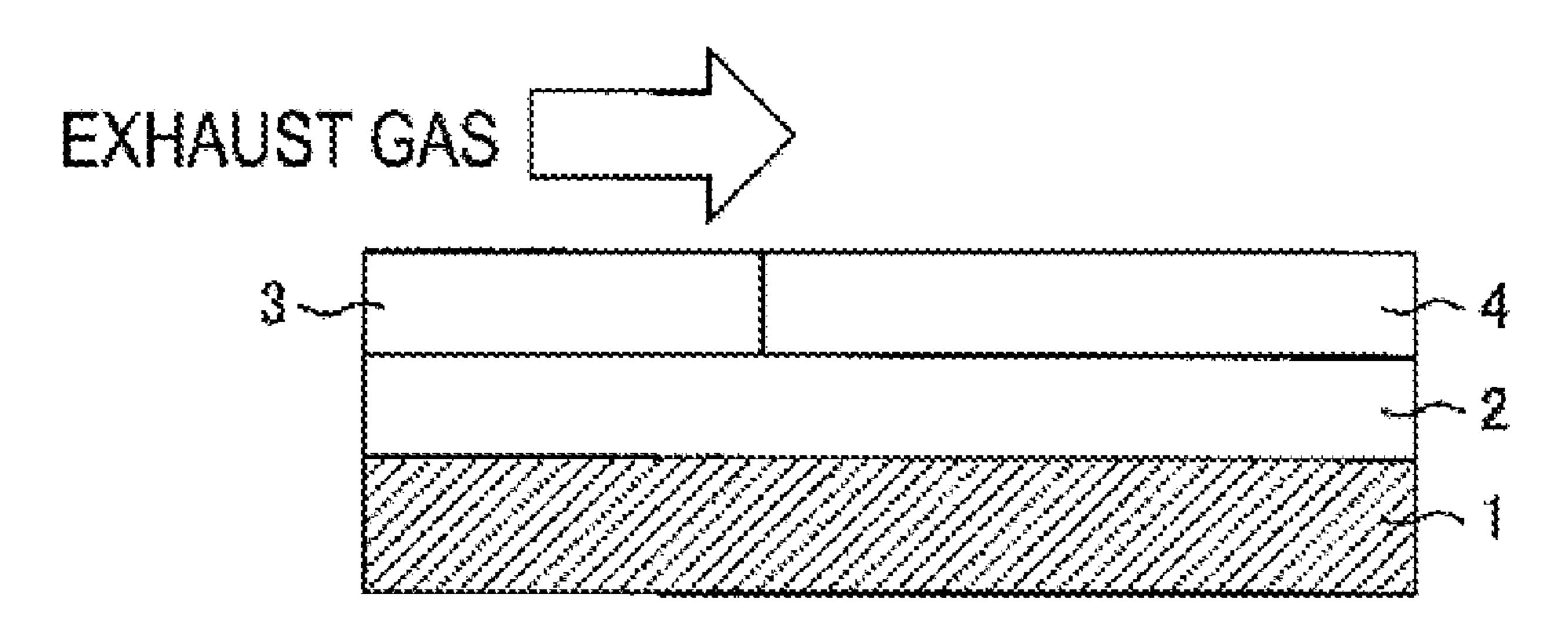
in order from an inflow side of exhaust gas to an outflow side of exhaust gas. The concentration of yttrium contained in the first region (3) and/or the second region (4) is higher than the concentration of yttrium contained in the region (2).
