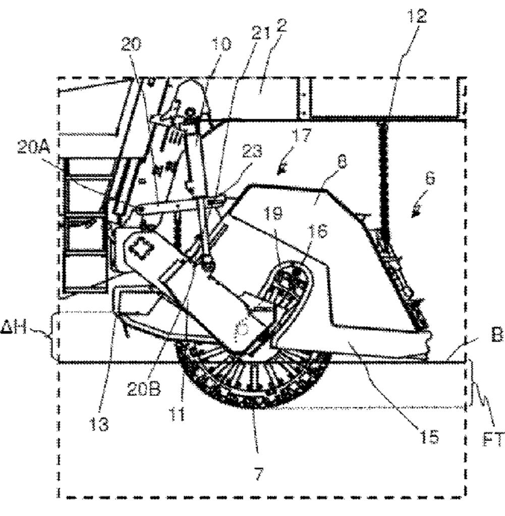
of the milling rotor housing relative to the machine frame depending on the milling depth.
