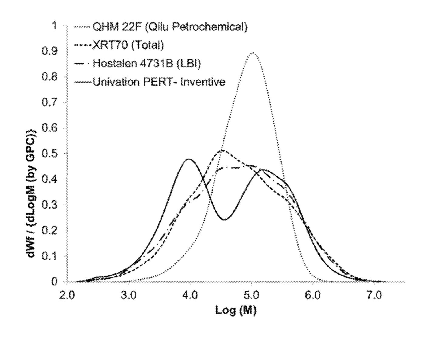
bimodal polymerization catalyst system includes a bimodal catalyst system of bis(2-pentamethylphenylamido)ethyl) amine Zirconium dibenzyl and either (tetramethylcyclopentadienyl)(n-propylcyclopentadienyl)Zirconium dichloride or (tetramethylcyclopentadienyl)(n-propylcyclopentadienyl) zirconium dimethyl in a 3.0:1 molar ratio; and a trim catalyst of (tetramethylcyclopentadienyl)(n-propylcyclopentadienyl)Zirconium dichloridedimethyl in heptane added to adjust melt.
