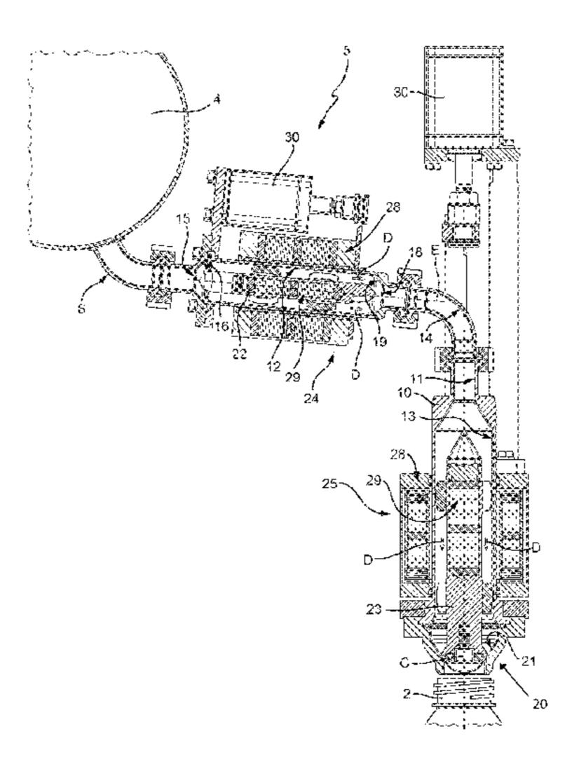
with a second pourable product having solid particles in suspension, in: the resting position, in which it defines a second maximum opening passage for the second pourable product; and a partial closing position, in which it defines a restricted passage for the second pourable product.
