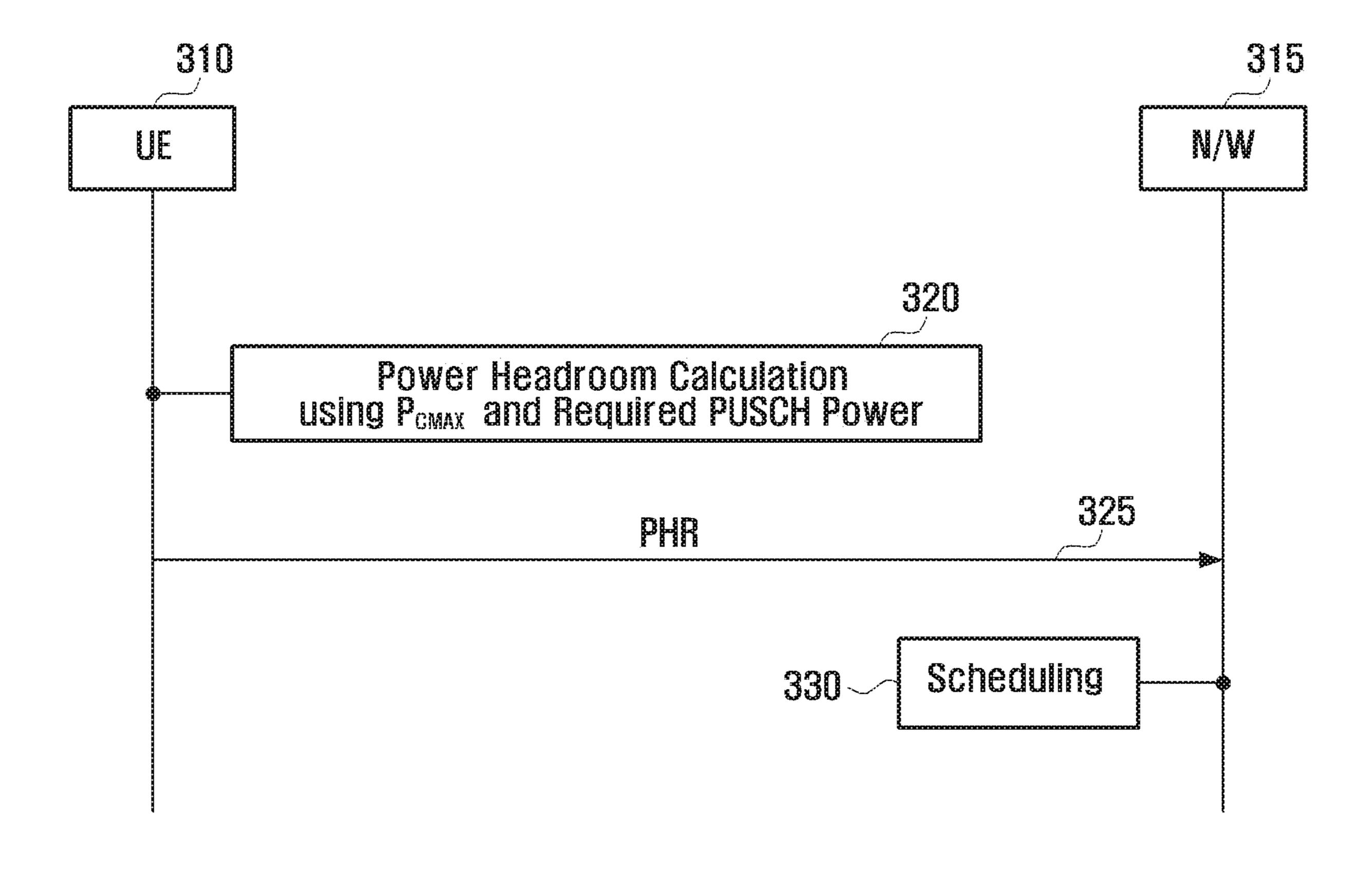
ENB estimates that the UE can be scheduled with 50 RBs/160AM based on the given PH modulation = 160AM, # of RBs = 50
