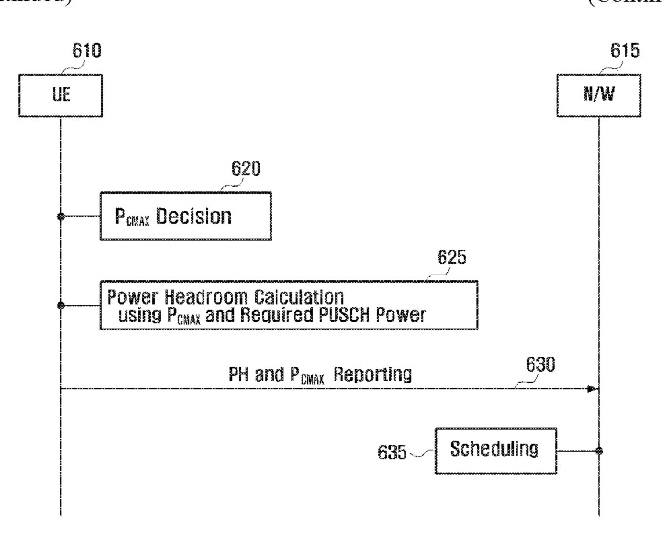
station in a scheduling process are also provided. A method for calculating a maximum transmit power in a constant manner regardless of a channel status is also provided.
