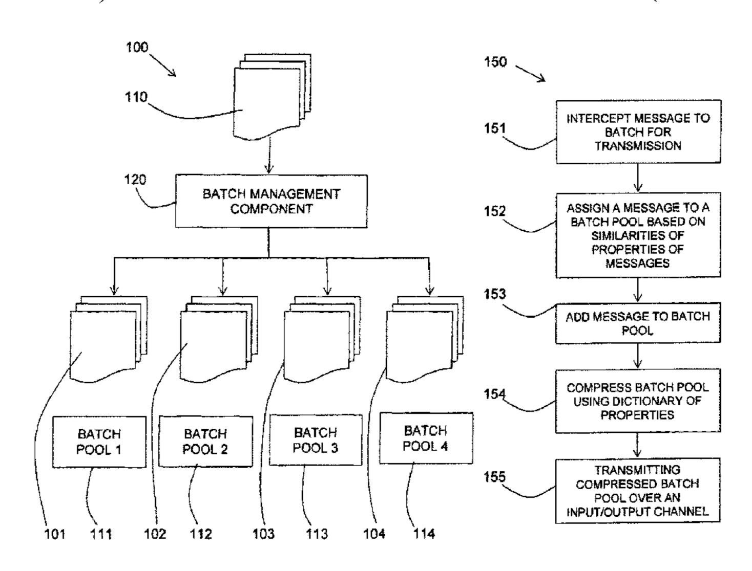
common to at least some of the messages in the batch pool. The compressed batch pools are transmitted over an input/output channel.
