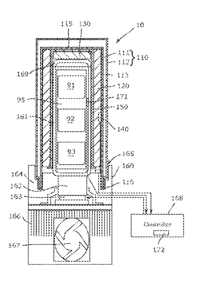
the thermally insulated container, and a storage space formed inside the heat-transferring body for storing a stored object so that the object can be freely put in and taken out.
