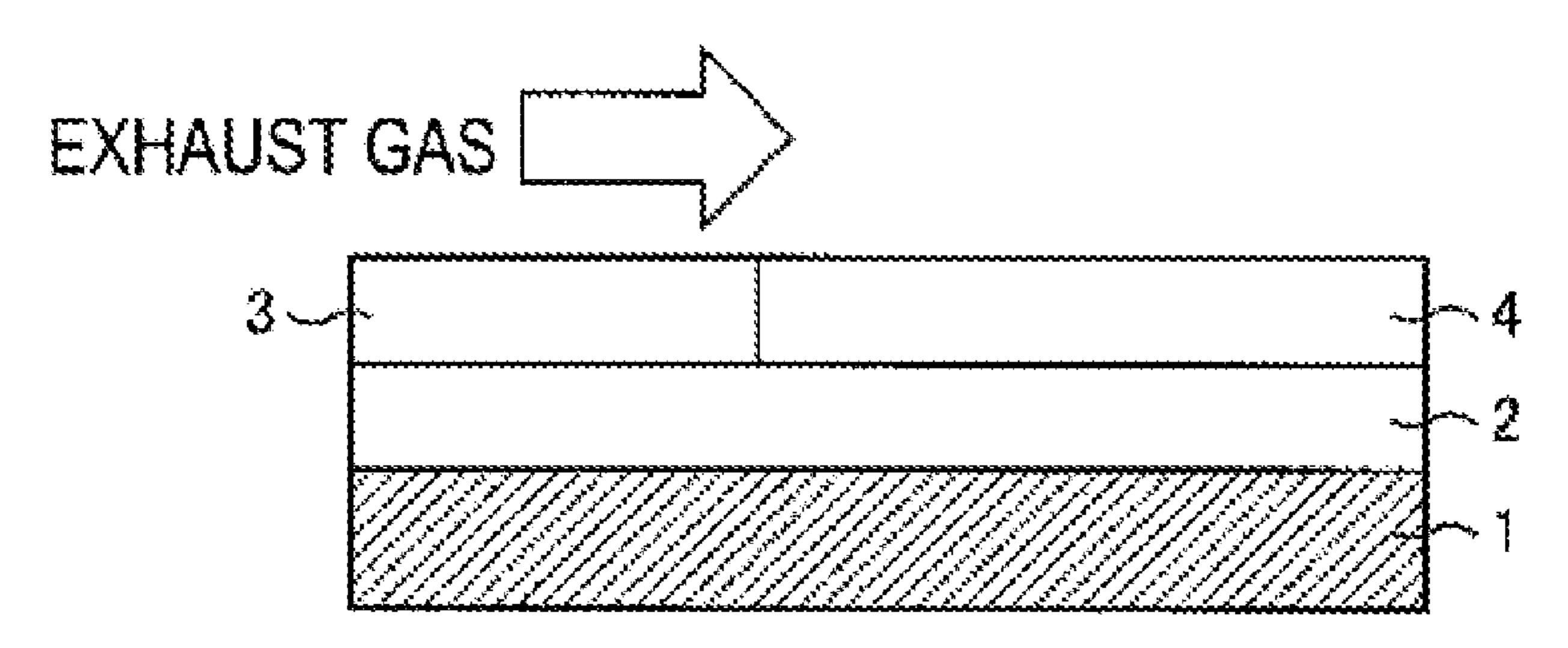
an inflow side of exhaust gas to an outflow side of exhaust gas. The concentration of neodymium contained in the first region (3) is higher than the concentration of neodymium contained in the second region (4).
