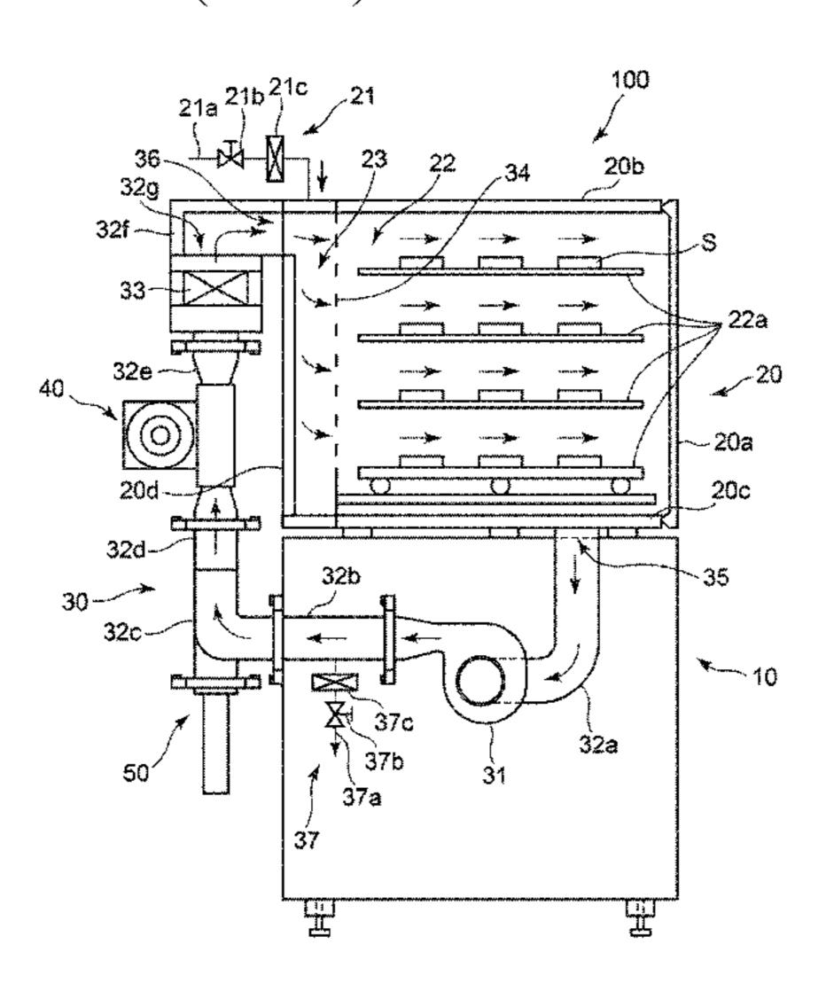
vaporizer can be directly supplied to the air circulated by the circulating means without passing through an air filter.
