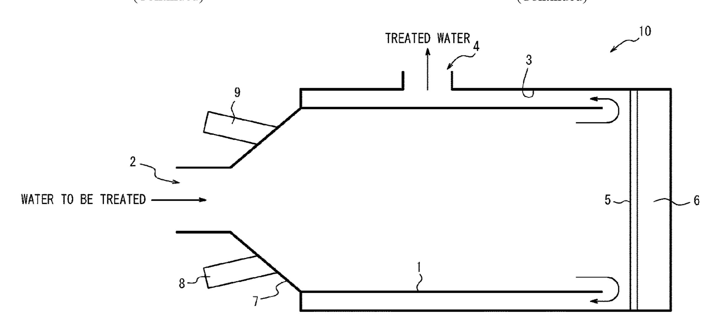
side of the flow channel from an inlet side, and irradiates the water to be treated flowing in the flow channel with ultraviolet light via a window portion toward the inlet side, the window portion being formed by a transparent member, wherein the flow channel includes a diameter increase portion, and the diameter increase portion is provided with at least one of: a cleaning device used to clean the window portion; and a sensor.
