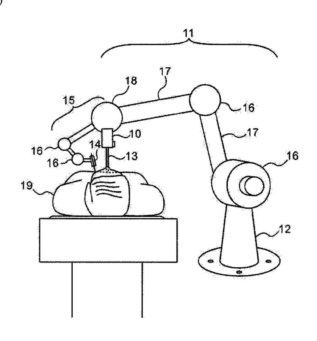
in breathing or coughing, the bone connector and base connection arm section, move together with motion of the patient's bone, while the pose of the end actuator relative to the patient is accurately maintained.
