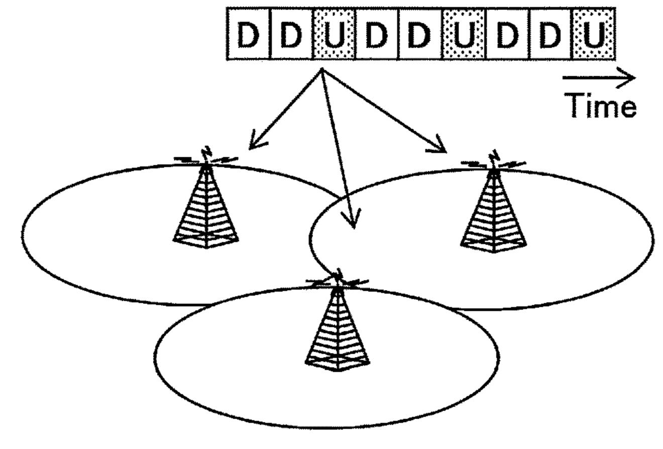
USE DL/UL PATTERN COMMON TO ALL CELLS (DL/UL IS PREDETERMINED)
