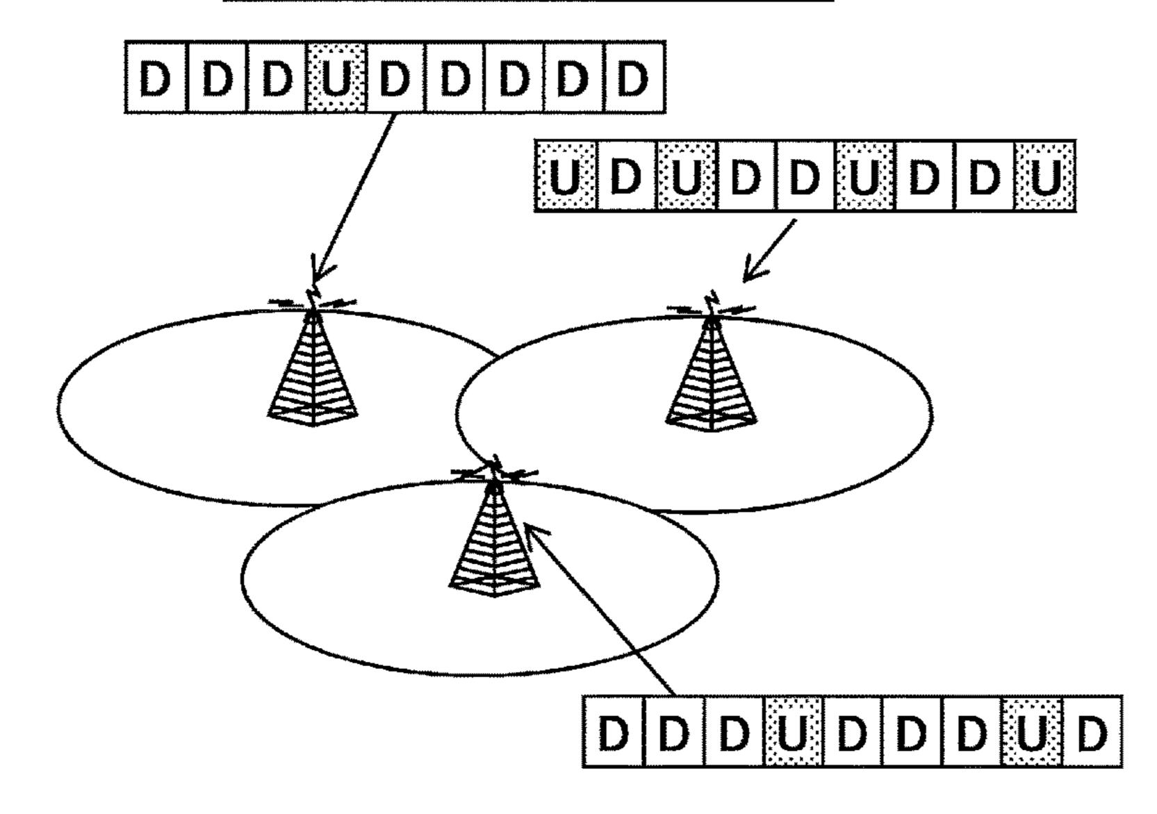
APPLY DL/UL PATTERN SPECIFIC TO EACH CELL (DL/UL IS VARIABLE DEPENDING ON REQUIRED TRAFFIC AT THE TIME)
