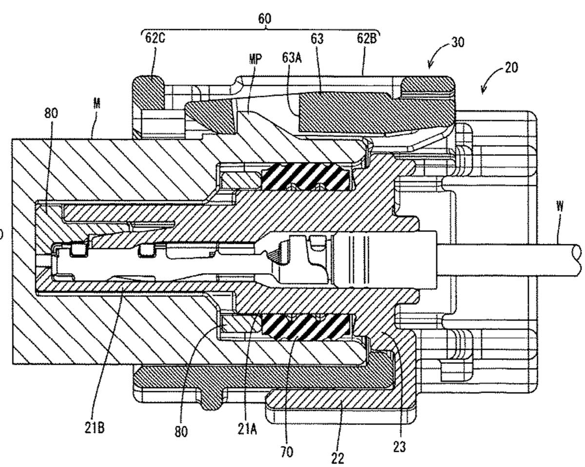
housing (20) and held connected to the mating housing (M) by releasing the first locks (50) at the time of separation from the mating housing (M).
