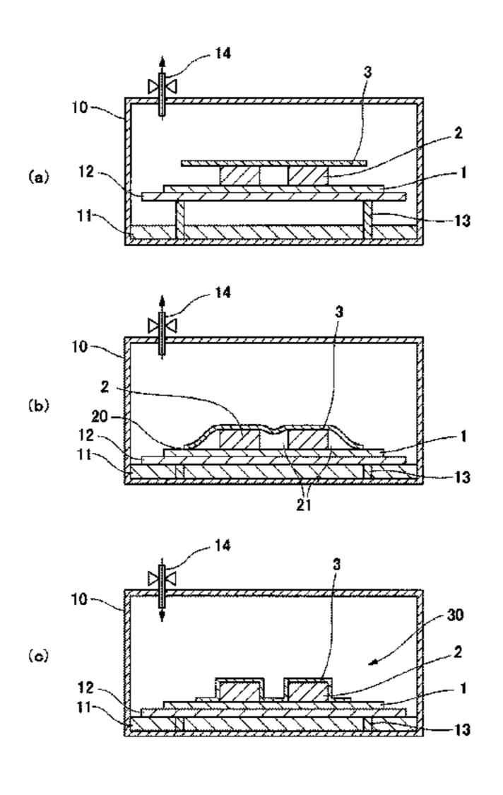
step in which the reduction of pressure within the chamber is released and the optical semiconductor element placement substrate is sealed by the film. The temperature  $T_2$  of the optical semiconductor element placement substrate when the reduction of pressure within the chamber is released is a temperature at which the film exhibits a tensile strength of 0.02-0.15 MPa and an elongation at break of 150-450%.
