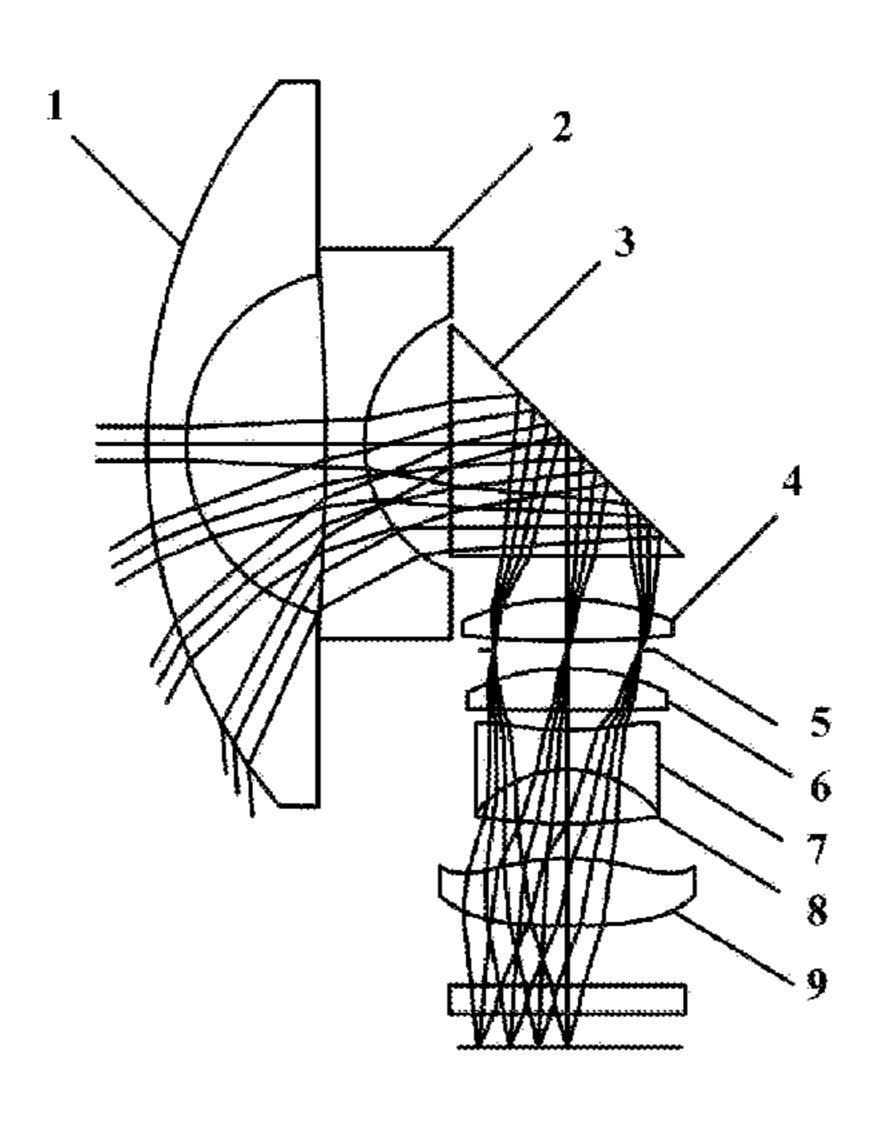
diaphragm is disposed between the third lens and the fourth lens. The camera lens and the imaging device of the present disclosure may not generate vignetting at the large field of view.
