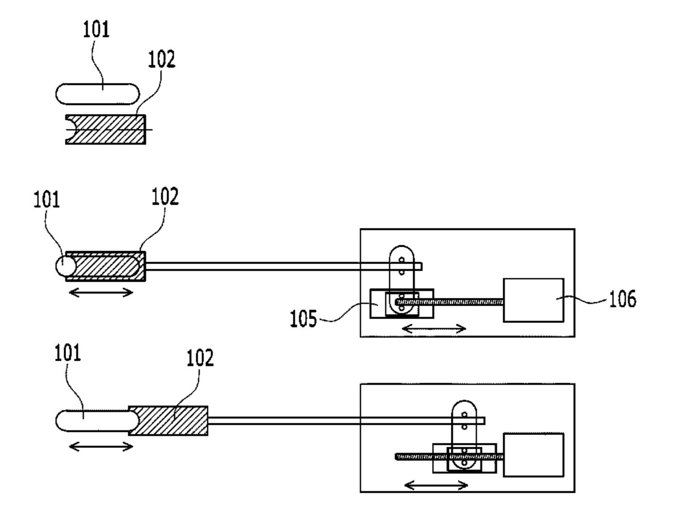
l/min, simultaneously with removing an measurement error caused due to inertia force of the suspended particles by automatically adjusting the cross-sectional area of the suction nozzle to suck the sample at the same flow rate as that of the stack gas in the stationary source emissions.
