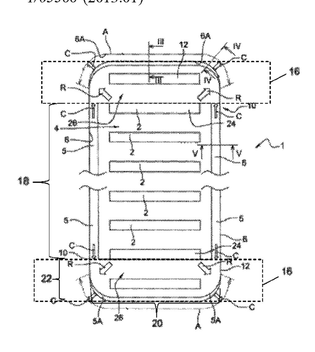
changes such that a radial dimension of the annular bead, measured in a median plane of the seal parallel to the annular shape of the seal, is smaller in the support part than in the connecting parts.
