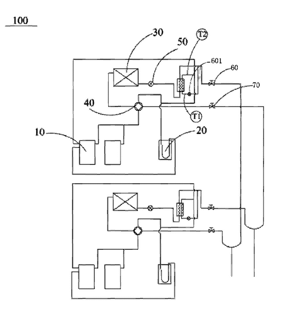
according to the result between the size of the average exhaust temperature of each outdoor unit and the size of the average exhaust temperature of the outdoor unit system, controlling an electronic expansion valve to actuate to make the average exhaust temperature of each outdoor unit to approximate to the average exhaust temperature of the outdoor unit system.
