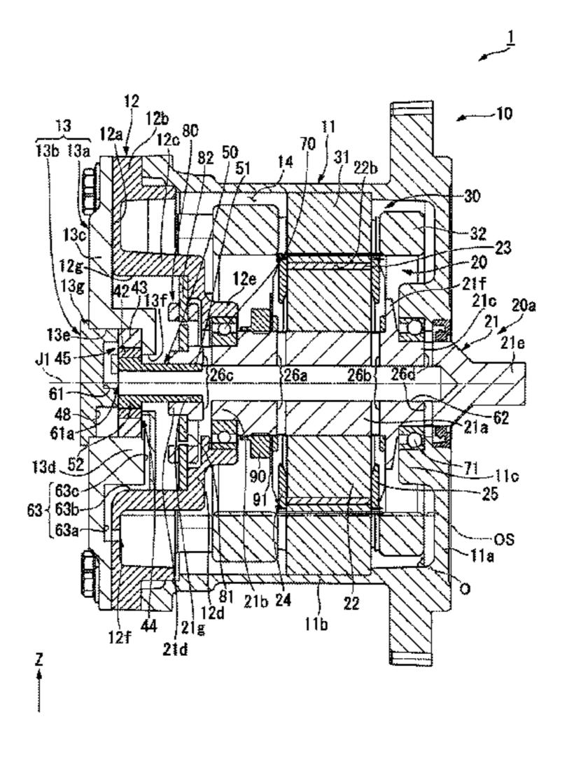
connect the second oil passage to the motor shaft. The second oil passage opens into the first oil passage at the end portion of the motor shaft.
