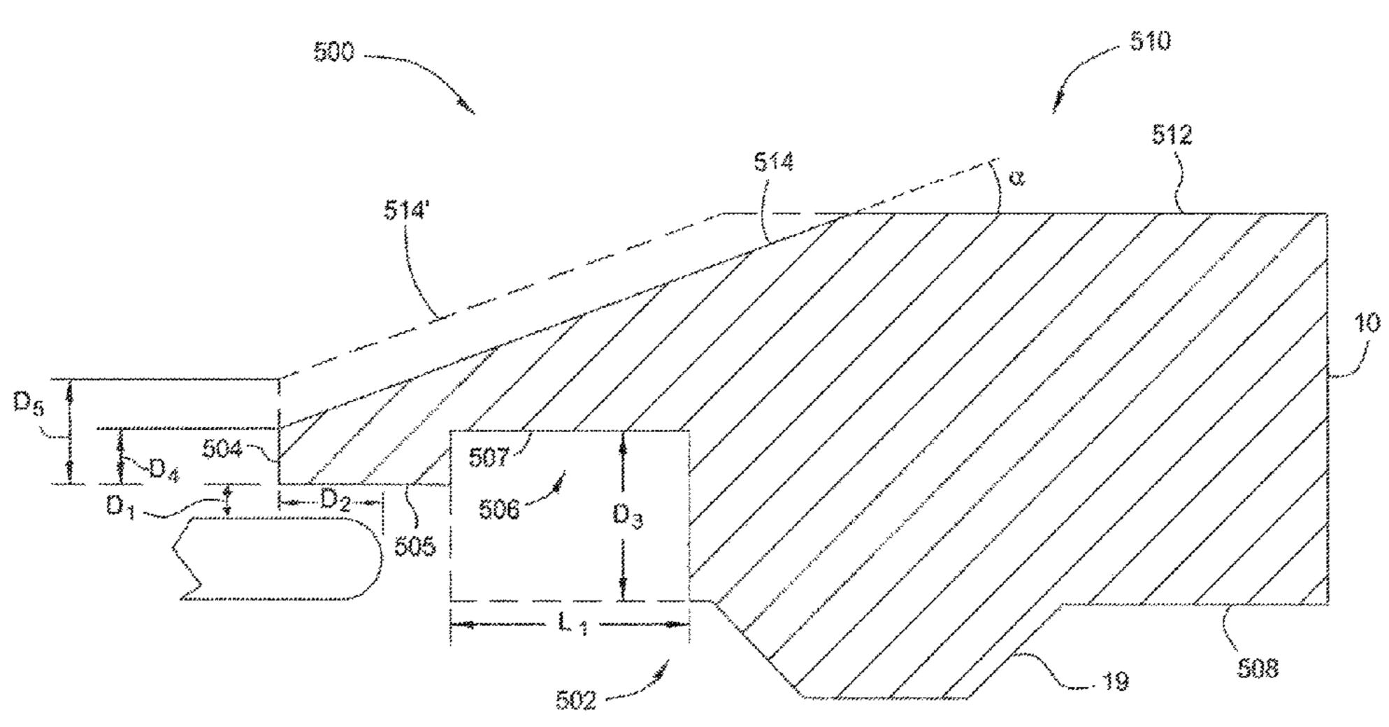
Another approach to adjusting the deposition at the edge of the wafer includes increasing or decreasing the inner diameter of the shadow ring. The material forming the shadow ring may also be varied to change the amount of deposition at the edge of the wafer.
