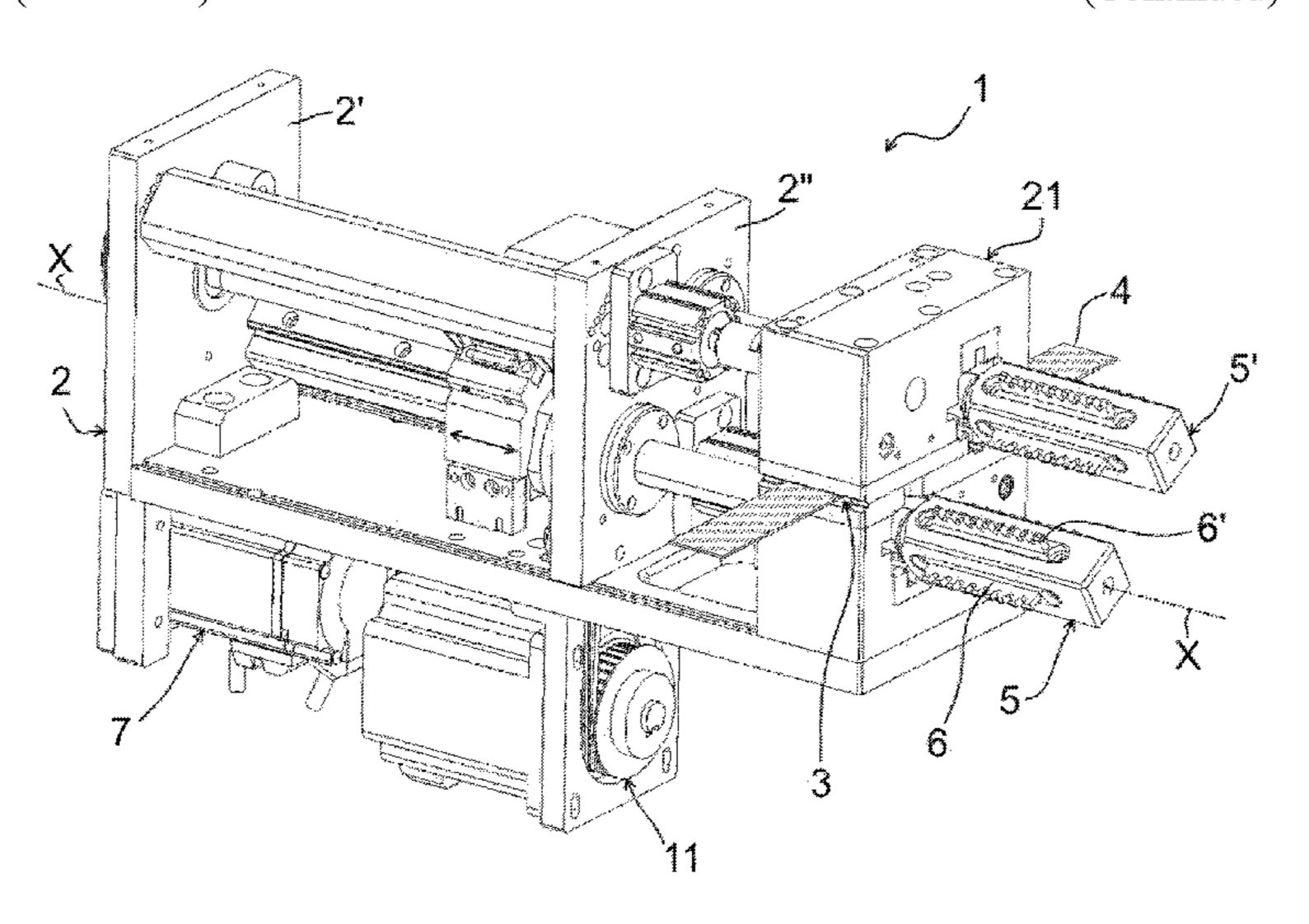
the guide, for example can rotate on itself, to selectively activate one of the broaching tools, i.e. to bring one of the tools into contact with the rule.
