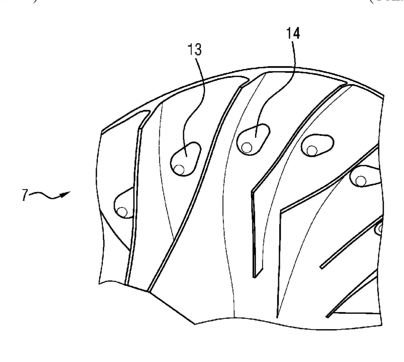
recess into a pear segment-shaped balancing mark. The invention furthermore relates to a turbocharger which comprises a compressor wheel that has one or more pear segment-shaped balancing marks.
