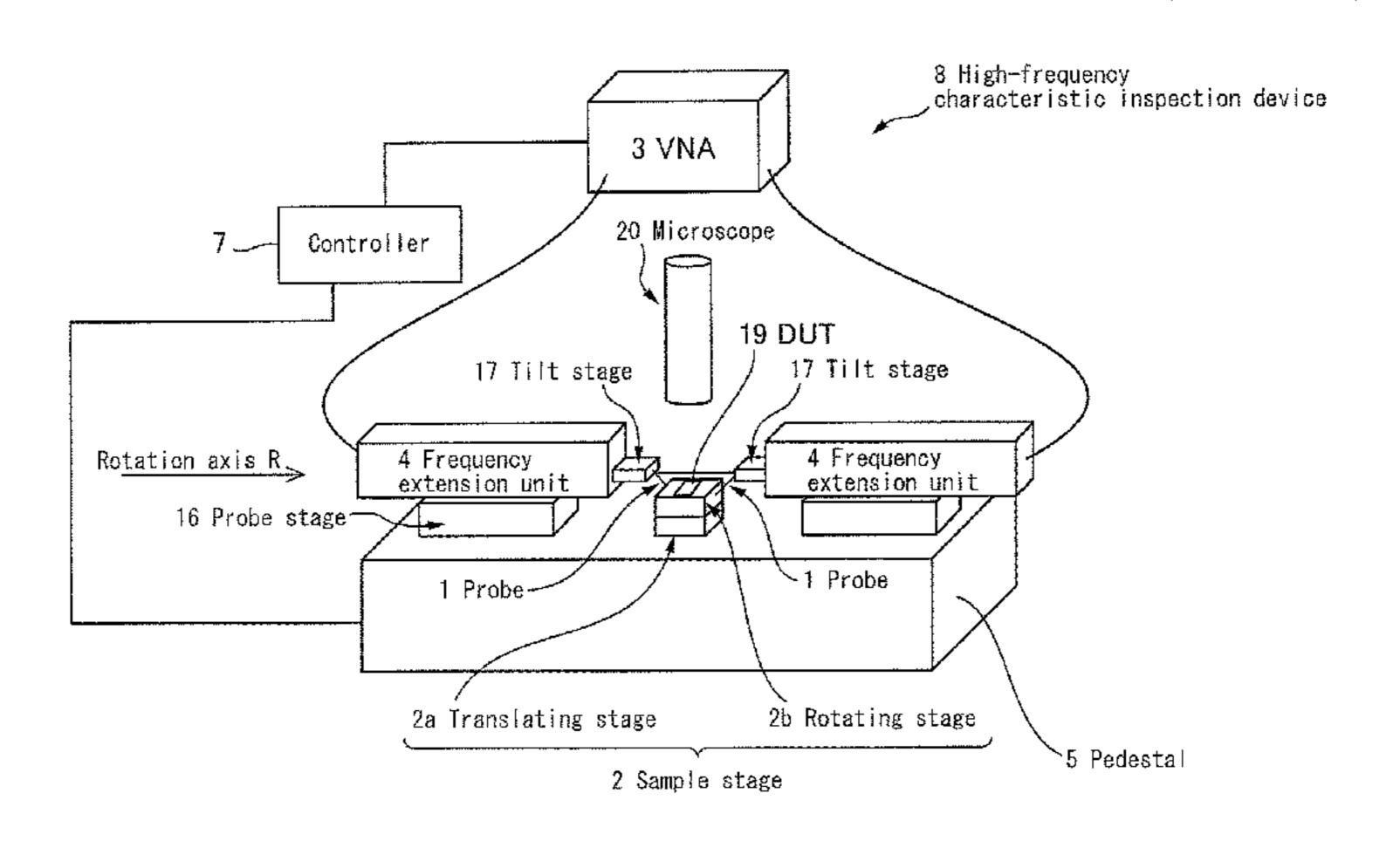
determining, based on a plurality of the S-parameters, a reference probe angle at which the reference line formed connecting the tip of the signal terminal and tip of the ground terminal is parallel with the conductor surface.
