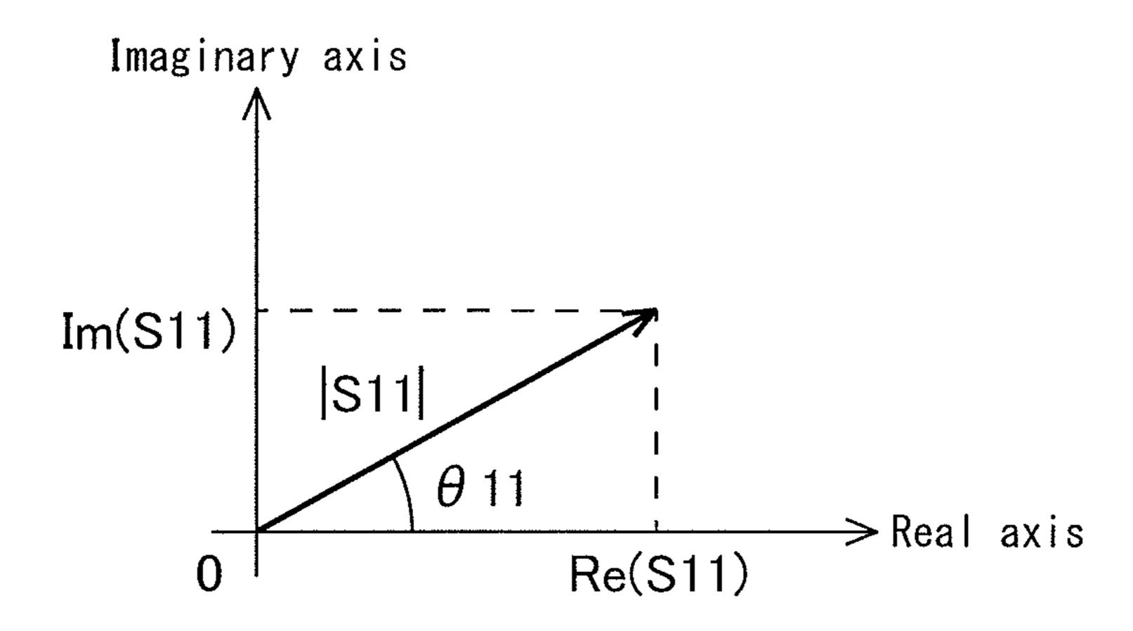
Reflection coefficient of reflected signal =  $|S11| \angle \theta 11$  (1)
