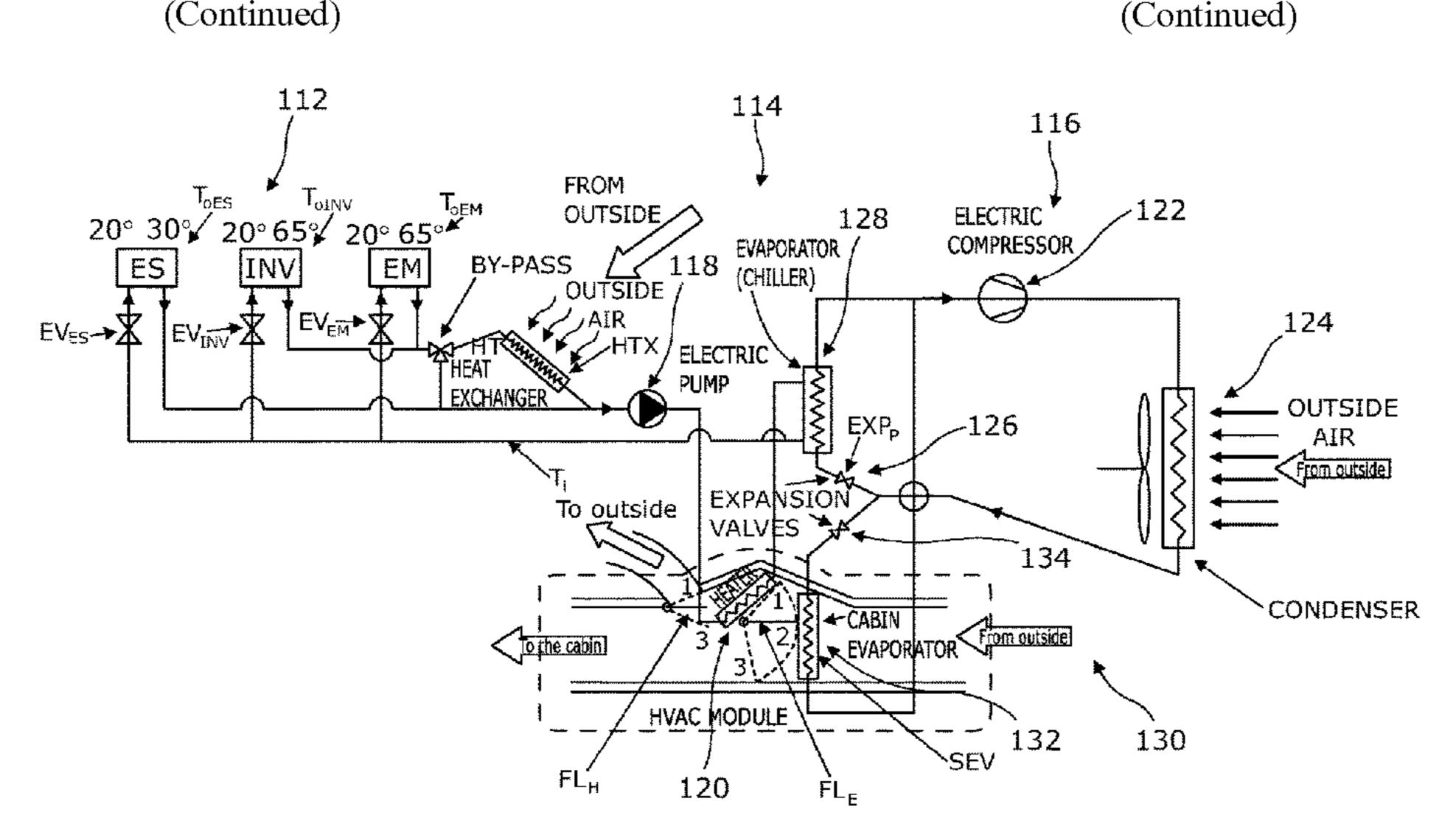
The chilled fluid flowing through the evaporator extracts heat from the fluid flowing around the first loop.
