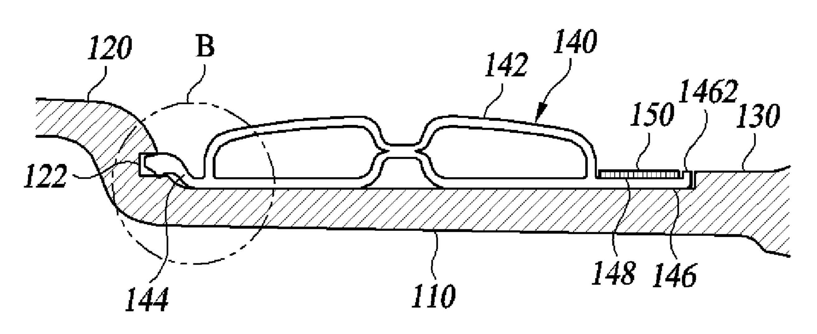
tube mounting groove; and a second flange protruding from a an opposite side of the tube body and having one end disposed adjacent to the second annular wall; and a fastening member surrounding one radially outer surface of the second flange between the tube body and the second annular wall along the circumference of the wheel rim, the fastening member pressing the second flange in a radially inward direction of the wheel rim.
