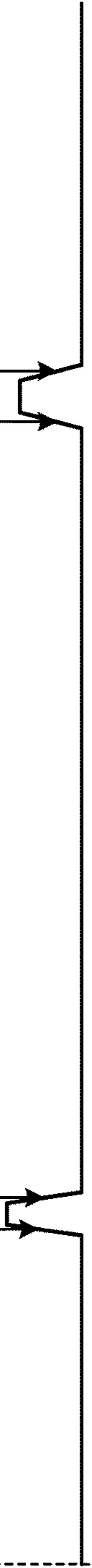
FIG. 7F OUTPUT SIGNAL OF RESET SIGNAL GENERATION UNIT
