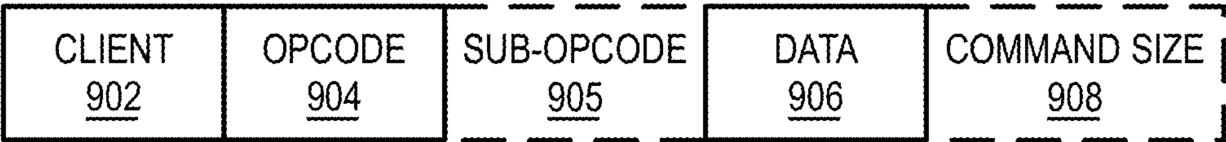
FIG. 9A GRAPHICS PROCESSOR COMMAND FORMAT 900
