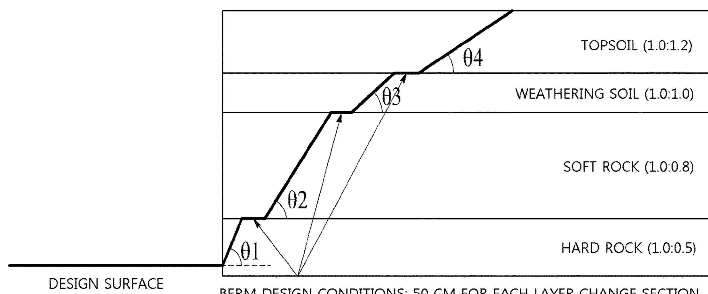
BERM DESIGN CONDITIONS: 50 CM FOR EACH LAYER CHANGE SECTION
