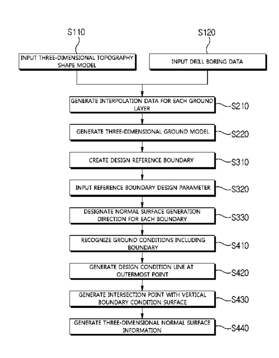
tion for each rock quality using the three-dimensional ground model, and sets the design condition.
