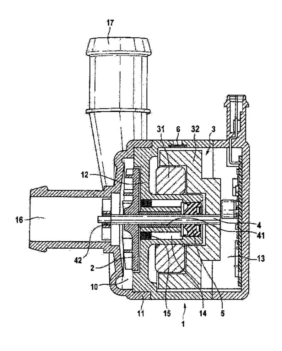
(32) is bell-shaped with an inner surface facing the shaft seal (5) and being fixed to the shaft seal (5) to axially overlap with the shaft (4). The motor chamber (13) has an opening to the atmosphere, which is closed by a liquid-tight pressure equalization membrane (6) that is permeable to vapor.
