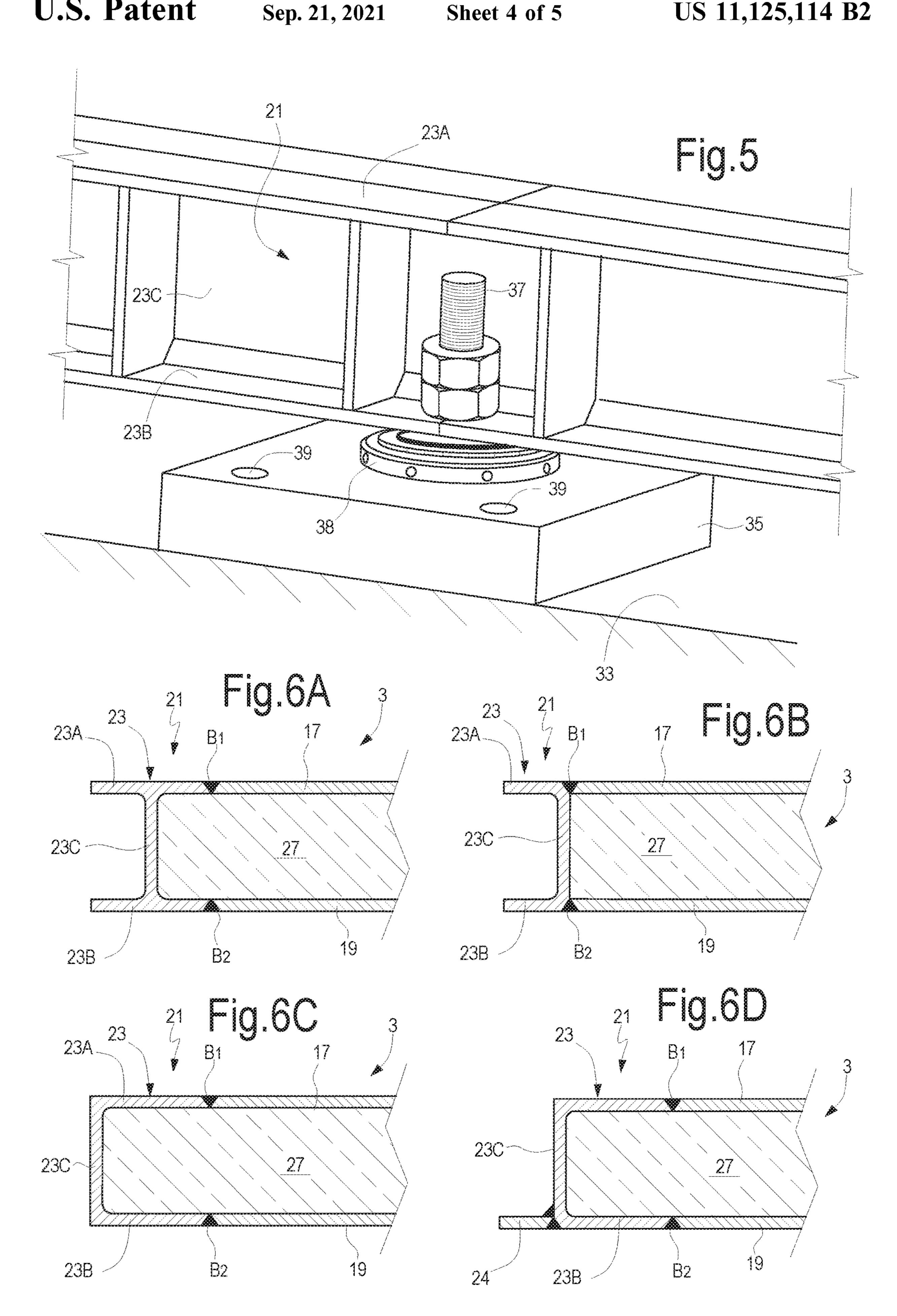
providing a base plate structure, comprising an upper metal plate, a lower metal plate, a frame extending peripherally along edges of Α the upper metal plate and lower metal plate; wherein the upper metal plate, the lower metal plate and the frame define a hollow volume introducing a flowable material in said В hollow volume causing the flowable material to set and adhere to the upper metal plate, the lower metal plate and the frame mount a gas turbine engine on the base plate structure
