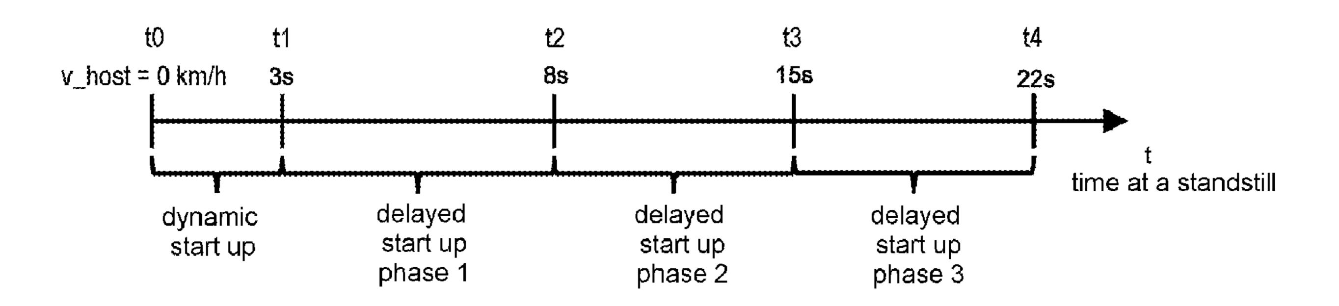
eration or the insertion of crawling phases. As a result of this, the driver is made aware of the automatic restart even after a long time at a standstill.
