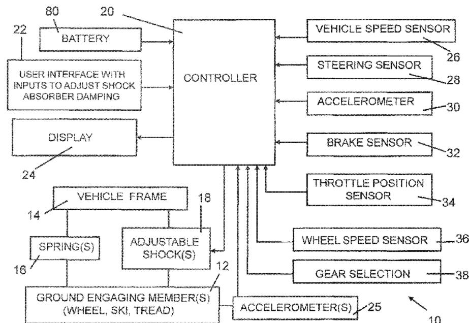
to adjust the damping characteristic of the at least one adjustable shock absorber based vehicle conditions determined by sensor output signals.
