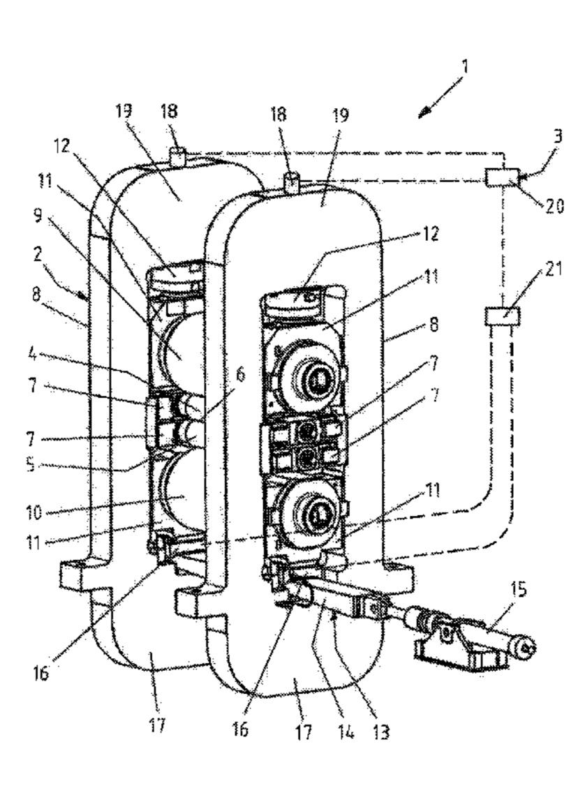
bearing unit (11) on a rack (8) of the roll stand (2). In order to enable an optimal active damping of vibrations in a roll stand (2) of this type with low engineering effort, the invention proposes that the supporting roll (10) is supported on the actuator (16) via at least one bearing unit (11) and that the actuator (16) is supported on a section (17) of the rack (8) either directly or indirectly via at least one component (14) of the readjustment device (13).
